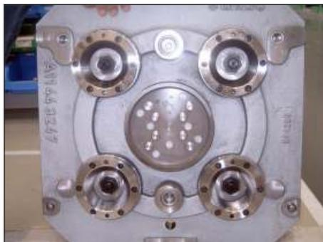
Coupling nipple plate in the fixture plate of a machine tool. The nipple plate is docked to the docking unit (figure above) and hydro-mechanical locked.
