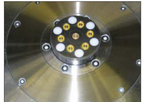
Coupling plate used for the transmission of hydraulic oil in the loading and unloading station of a fixture plate. The six coupling elements are coupled pressurised.
