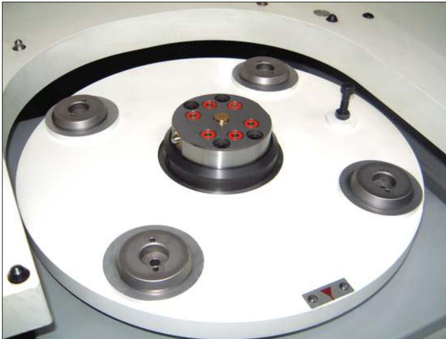
**Application example:** six-fold coupling system with self-locking, two pairs of lines are each pressurised double-acting and two lines are used for pneumatics. The fixture pallet does not have to be clamped in the loading station in order to absorb the coupling forces. For this purpose, the system has the self-locking function.
