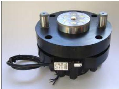
Docking station with six coupling points, pressurised coupling; In order to dock the coupling plate, it is raised by an integrated hydraulic cylinder. An electronic sensor queries the position
