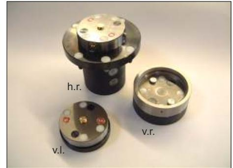
Coupling system with hydro-mechanical locking and two coupling points:
